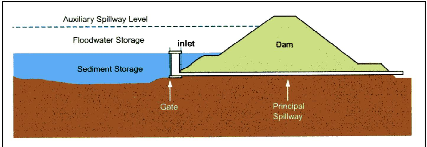
This cross section of a dam shows the concrete inlet in front of the dam connected to the principal spillway pipe (extending through the dam). When water reaches the opening at the top of the inlet it spills over and goes through the pipe controlling the level of water in the lake. Some inlets also have openings in the side of the tower.
