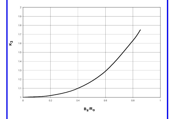
RATIO OF MAXIMUM BOUNDARY SHEAR IN BENDS TO MAXIMUM BOTTOM SHEAR IN STRAIGHT REACHES
