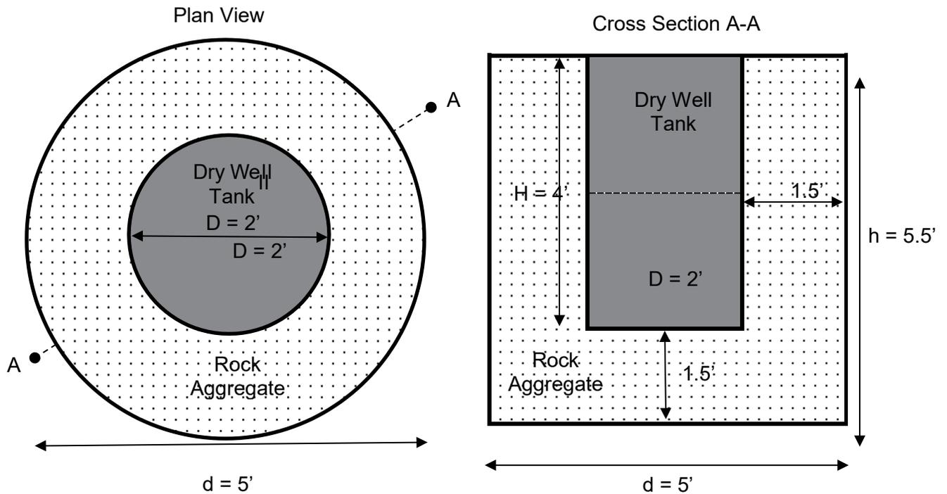
On the following page, the rock aggregate volume (RV) provided by the design will be calculated to determine if provided volume meets the required minimum volume required to treat the drainage area.
