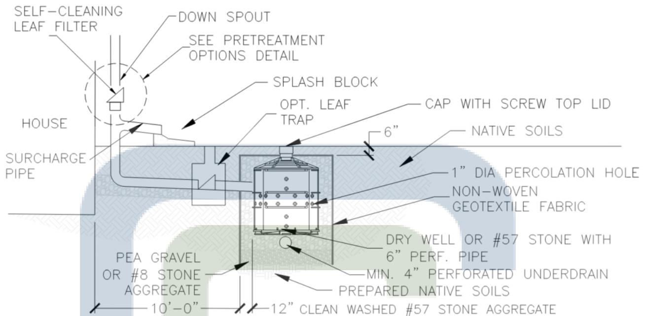
**TYPICAL COMPONENTS OF SEEPAGE TANK DRY WELL
