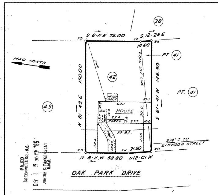
0 40 80 /20 SCALE: 1" = 40' FEET NOTE: 5' DRAINAGE & UTILITY EASEMENT ALONG ALL SIDE & REAR LOT LINES.
