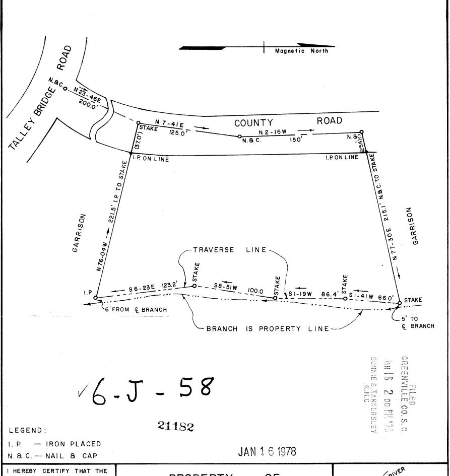
I HEREBY CERTIFY THAT THE RATIO OF PRECISION OF THE FIELD SURVEY IS I / 5200 AS SHOWN HEREON AND THE AREA WAS DETERMINED BY DMD METHOD OF AREA CALCULATIONS.
