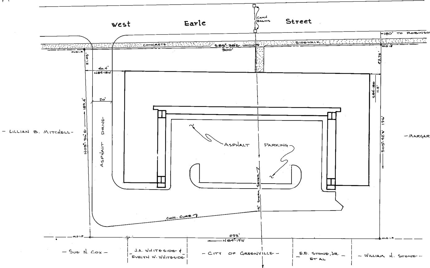
THE UNDERSIGNED CERTIFIES THAT THE BOUNDARY FOR THE PROPERTY WAS DRAWN FROM AN ACTUAL SURVEY DATED AUGUST 16, 1976 MADE BY ME AND THAT THE COURSES AND DISTANCES ARE TRUE AND CORRECT; THAT THE BUILDING AND IMPROVEMENTS LOCATED THEREON ARE ACCURATELY LOCATED; THAT THE BUILDING AND IMPROVEMENTS DO NOT ENCROACH OR PROJECT OVER THE BOUNDARY LINES.
