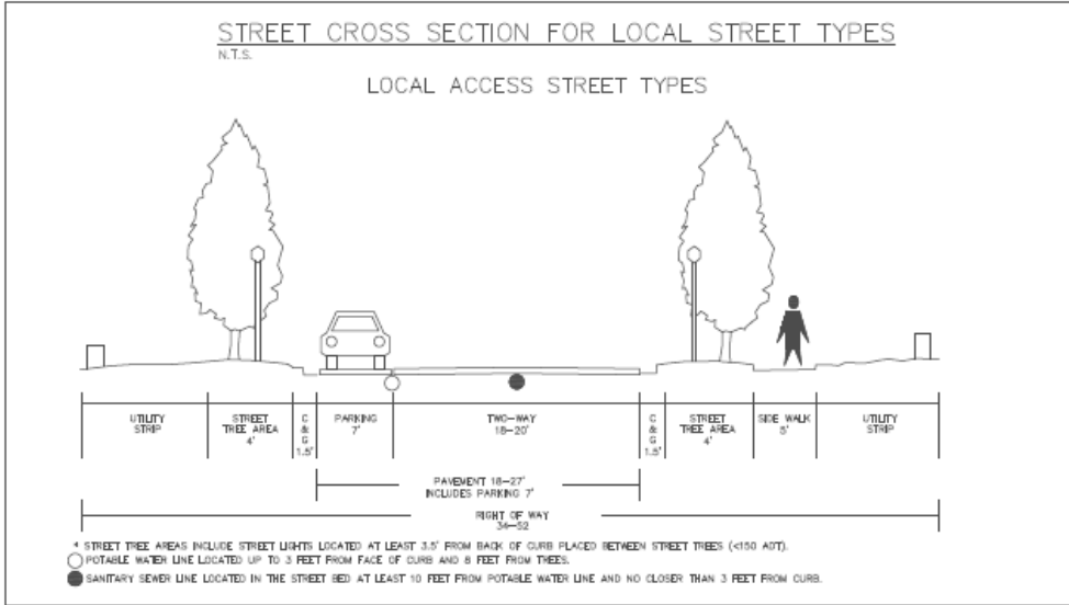
Exhibit 13.1 Street Cross Section for Local Street Types.
