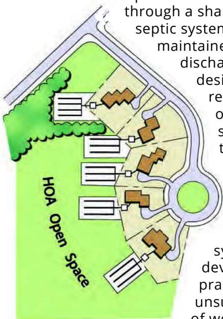
HOA open space used as shared drainfields for individual septic systems. Illustration from Growing Greener: Conservation by Design by Randall Arendt.
