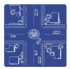
**Design characteristics:** Two-lane roads, no other traffic control needed, trucks may turn in front of circle, circle diameter 15'-20'
