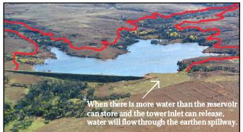
The red line on this photo indicates the extent that water can back up in the flood pool upstream before it starts flowing through the earthen spillway. This is where flood water is stored while it is slowly released through the principal spillway pipe.
